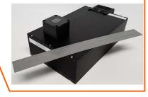
supports excitation frequencies up to 400 Hz (via an external yoke)
