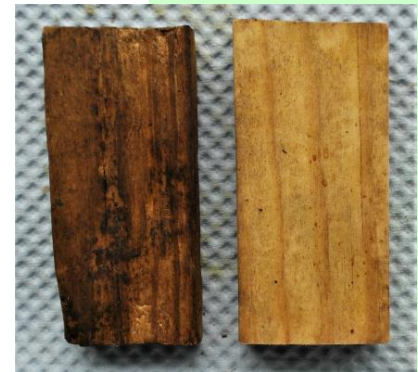
Jaw – untreated and treated after 16 weeks of exposure with conioophora puteana
