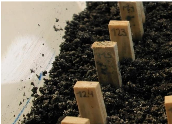
Soft rotting test according to DIN V ENV 807, 32 weeks trial period, determination of the mass difference
