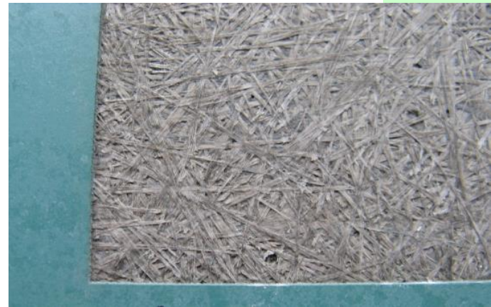
selective removal of layers of a glass-fibre reinforced composite (grp)
