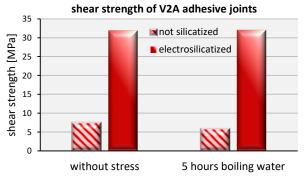
Example: Improving the adhesion of stainless steel adhesive joints by electrosilicatization and use of silane coupling agent – unstessed & after boiling water treatment;
