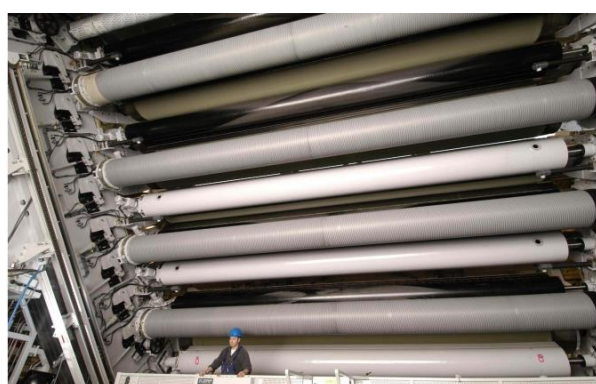
composite roller of a dryer section of a paper machine (photo: xperion)
